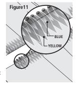
▲ CAUTION: BEFORE ATTEMPTING TO IGNITE YOUR BARBECUE, FOR YOUR SAFETY PLEASE CONDUCT A VISUAL CHECK TO ENSURE THAT THE BURNERS ARE ALIGNED WITH THE VALVES CORRECTLY, THAT ALL CONNECTIONS BETWEEN THE GAS SUPPLY LINE AND THE BARBECUE ARE TIGHTENED, AND FINALLY THAT A COMPLETE LEAK TEST IS COMPLETED.
