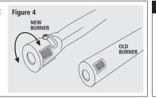
Install the new burner into your barbecue. Make sure the opening on the front burner (A) is properly aligned with the gas valve.
